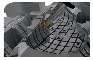
5 axis machining of a mold with TopSolid'Cam.
