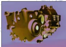
THE SINTERED POLYSTYRENE GEAR BOX AFTER WAXING FOR PRECISION CASTING.
